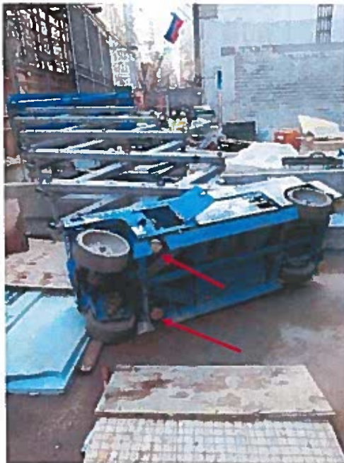
Photo 5 Accident scene showing toppled lift with outriggers not deployed.
