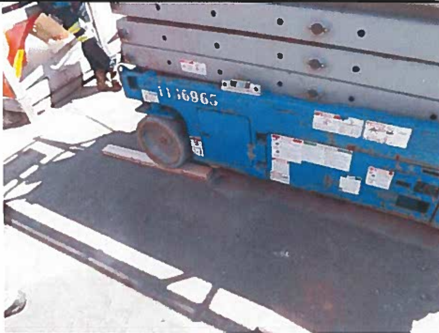
Photo 8 Left front wheel on a 2 x 4 during the test of the tilt sensor.
